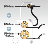
**2 torches, 2 integrated wire feeder + 1 Spool Gun** - The T3 GYS AUTO is a multifonctional and flexible machine designed to weld 3 different type of wire or diameter at the same time. It's saving time by avoiding disassembling the torch and changing the wire reel for another job.
