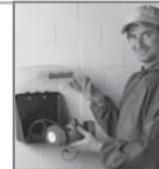
Masks in use must be stored in their appropriate hygiene storage boxes, in special storage cabinets or other suitable containers in order to protect them from dust and vapours. Masks may only be stored when they are completely dry. They may not be exposed to direct sunlight and must be kept away from heat sources. Never immerse masks in solvents.
